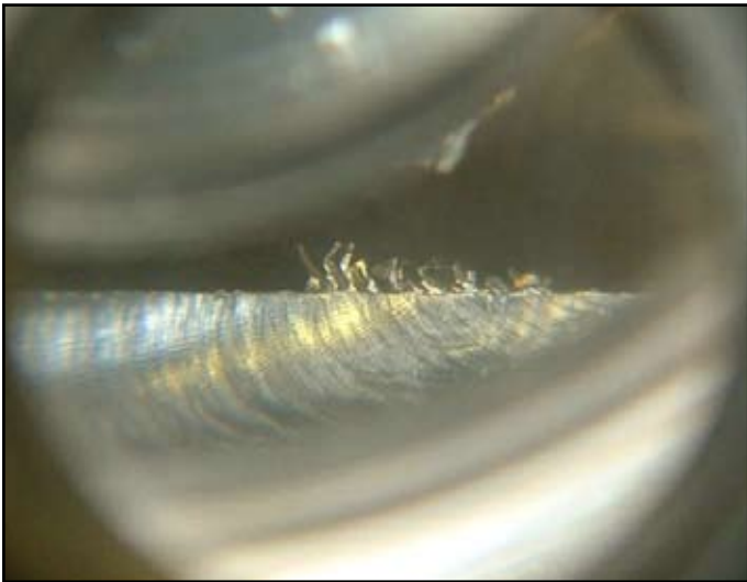
Stainless steel; fine milled burrs, easily missed by hand and eye especially with 0.1mm burrs. 10x
