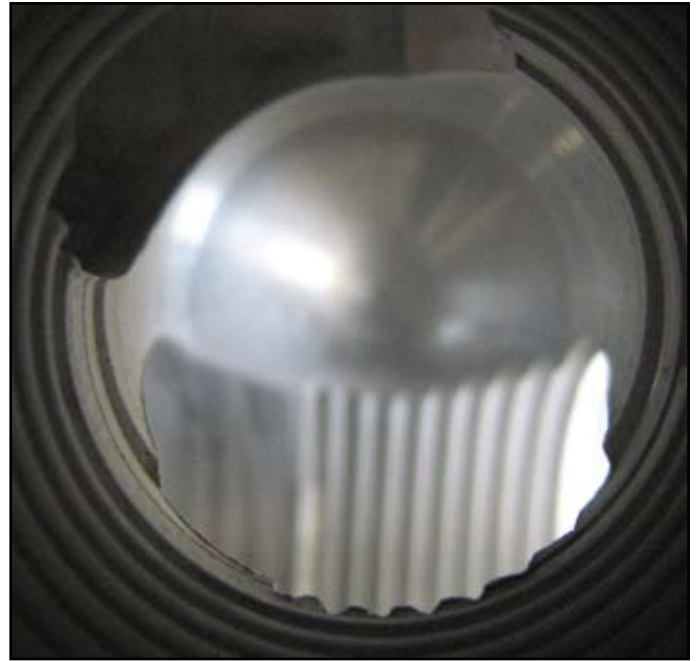
Aluminium manifold block; cross hole into thread, time consuming by hand. 3x
