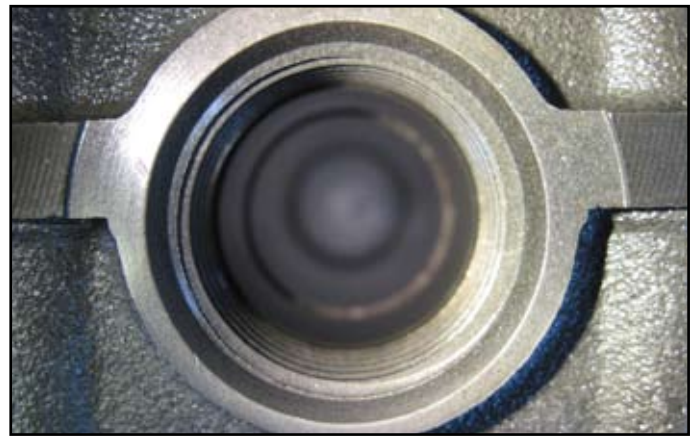
Cast iron; the thin leading edge of threads are burnt back and angel hairs removed. 1x
