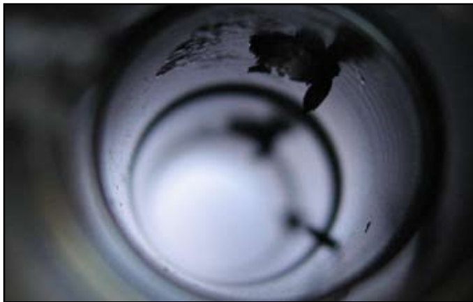
Steel, a typical crown burr and cap left after drilling. 2x
