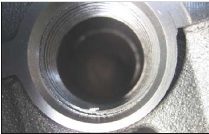
Cast iron; the thin leading edge of threads are burnt back and angel hairs removed. 1x
