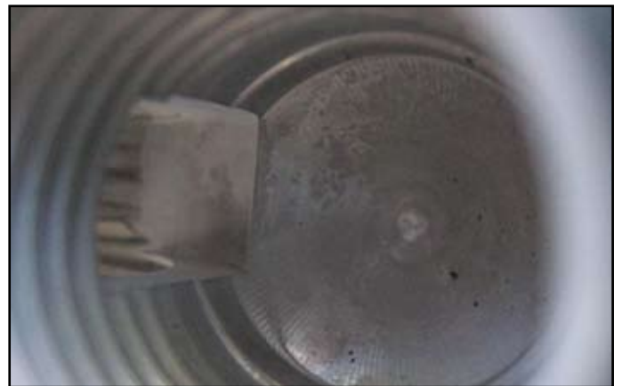
Aluminium manifold; removing the last piece of material pushed away from milling cutter. 3x
