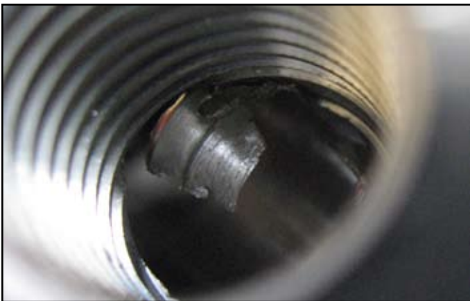
Aluminium manifold; removing the last piece of material pushed away from milling cutter. 3x
